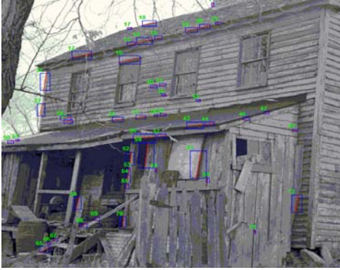
Figure 3. An example of the detected valid edges on an image from Set #7.
